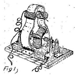
This is one of the most effective of the small simple motors. I have made because, being of the tripolar type, it is self starting. It cost very little to make, as the magnet and armature was made from a stout tin canister, and the rest, with the exception of the
